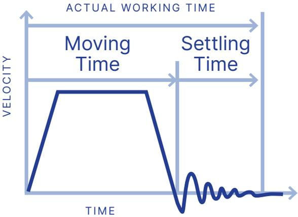
Manufacturing processes increasingly demand shorter cycle times for improved throughput, which in turn, requires higher speed and acceleration rates from the robot. But as speed and acceleration increase, so does vibration in the robot arm. As a result, the ratio of settling time to the overall cycle time increases, reducing throughput and precision.
